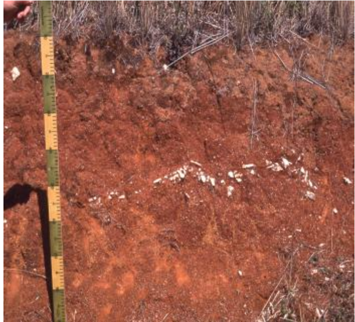
Figure 5. White gravel from a colluvially disturbed quartz vein, now buried in the lower B horizon
