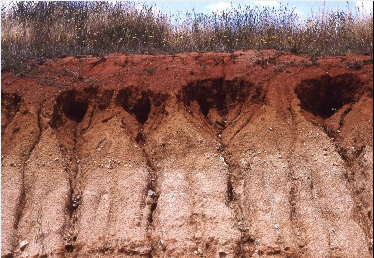
Figure 19. A red Burringong soil in a roadside batter 2 km from Young, where the aggregates in the A and upper B horizons appear less prone to slaking than those in the lower B horizon, presumably associated with the decreasing organic matter content down the profile. The pale weathered granite in the C horizon still retains enough rock fabric to stay cohesive and resist structural breakdown.
