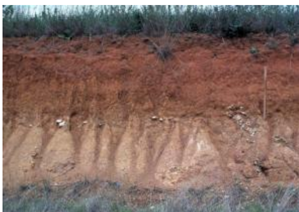
Figure 3. Colluvial action in the past has spread gravel remnants of this quartz vein on top of the saprolitic pallid clay (note metre rule on right)
