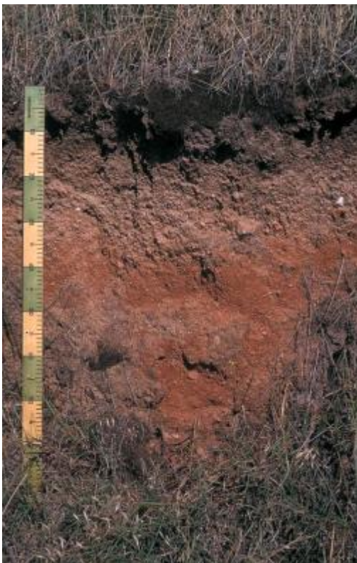
Figure 6. A gravel-rich A2 horizon above a less gravelly but more clayey and (typically) weakly structured B horizon on an upper slope 6km north east of Young
