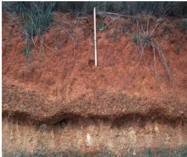
Figure 7. A band of ironstone gravel 30-50cm thick resting on pallid clay; the gravel is below the weakly structured red lower B horizon in this road cutting 4km north of Young
