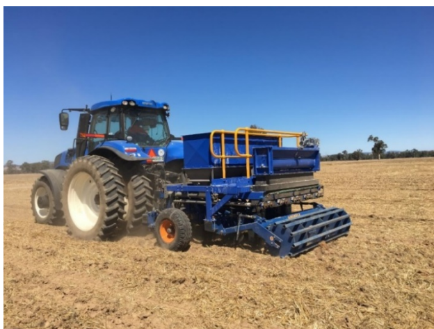
Figure 5. 3-D Ripper, designed and fabricated by the NSW Department of Primary Industries
