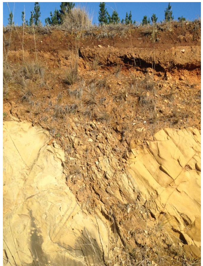
Figure 10. Roadside cutting near Ashton Creek showing interbedded sandstone/ shale/ sandstone
